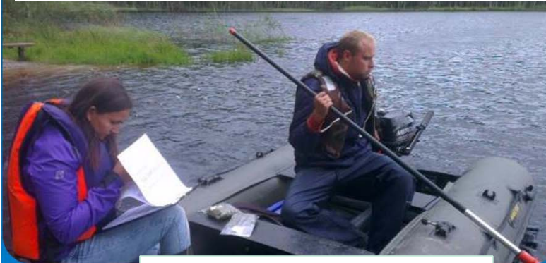
Macrophyte sampling by using a rake (<4m depth) or scraper (>4m depth)
