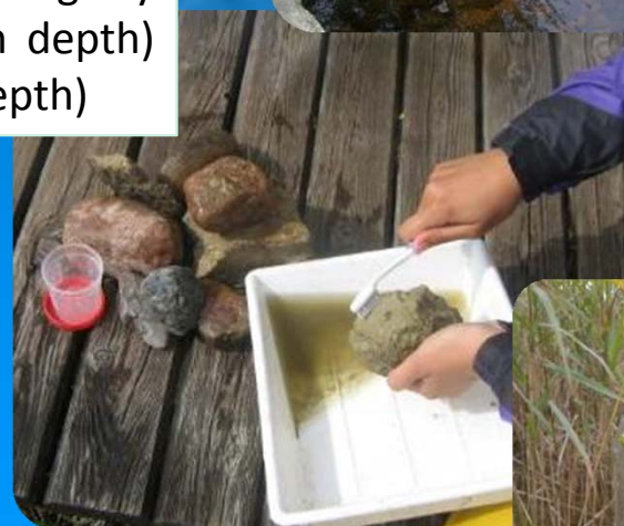
Diatom sampling from stones with toothbrush, from macrophytes using a jar
